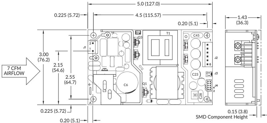
In the case above, the power supply requires forced air of 7CFM in the direction indicated by the arrow. The cross sectional area is:-
