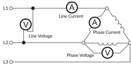
The line current is higher than the phase current by a factor of the square root of 3 (1.732). The reason for this difference in current is that current flows through different windings at different times in a three-phase circuit. At times, current will flow between two lines only, at other times current will flow from two lines to the third.
