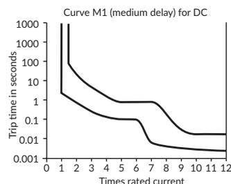
The important issues are the same; ensuring that there is adequate time delay to prevent tripping during the initial inrush and the breaking current if it is being used in a battery application.
