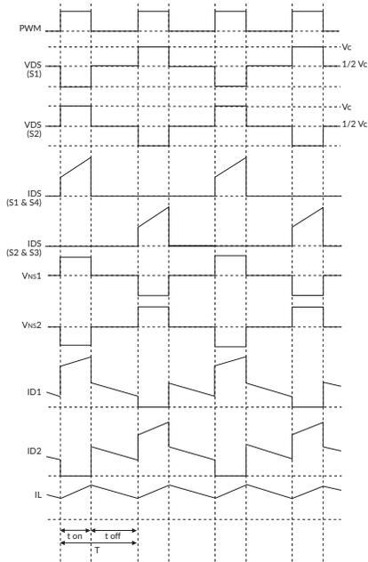
This topology will provide double the output power for the same primary switching current, but increases the complexity of switching element drive circuits, compared to the half bridge.
