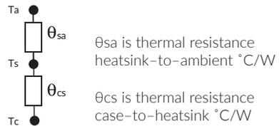
Thermal resistance to the flow of heat from the power module to the ambient temperature air surrounding the package is made up of the thermal resistances of the case to heatsink and heatsink to ambient interfaces and can be added together to give an overall thermal resistance from power module to ambient  $\theta_{ca}$ .
