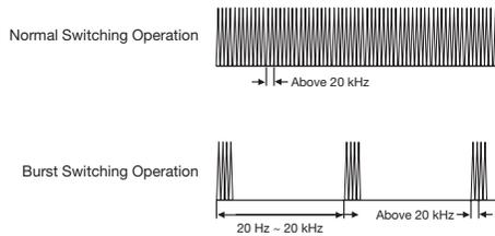
Steps are taken to mitigate audible noise such as varnish impregnation of transformers and other wound components, changing ceramic capacitors to film types in key areas to avoid piezo electric effects and controlling burst mode frequency to avoid the areas most sensitive to the human ear (2kHz–4kHz). These steps may not eradicate audible noise under all conditions but go a long way to minimize the effects.
