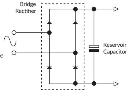
The bulk capacitor is charged during the conduction angle and is discharged slowly by the power stage of the power supply ( $V_{CAP}$ ). As soon as the input sine wave voltage falls below the bulk capacitor voltage then the diode in the bridge rectifier is reverse biased and no current flows until the incoming rectified sine wave is once again higher than the bulk capacitor voltage. The conduction angle is typically 2-3ms.
