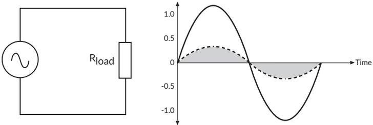
The phase angle between voltage and current is zero, the two elements are in phase.
