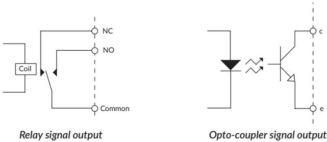
A benefit of isolated signals is that they can be combined into a single warning when using multiple converters in series or parallel combinations and can be referenced to a common signal ground for the end equipment interface, regardless of positive or negative output configuration.
