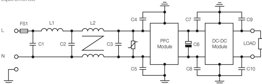
**Example: schematic for AC input systems**
