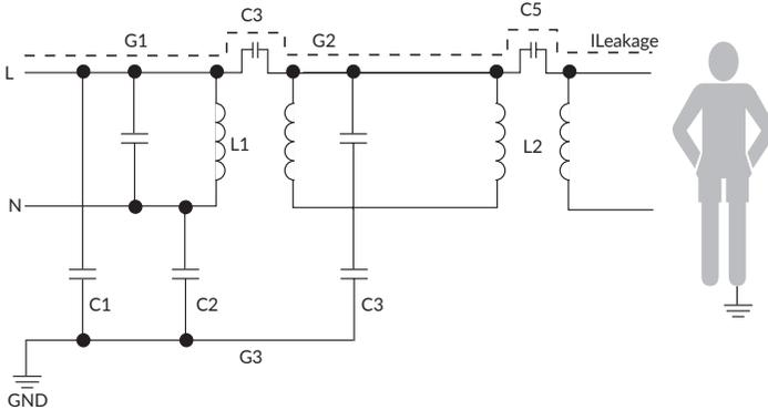
**Simplified model for power system with secondary DC-DC isolation.**
