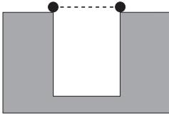
**Clearance is the distance between two points through air**
