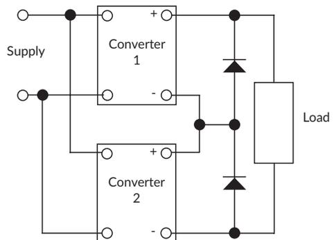
Power supplies with constant current or constant power limit are recommended for series operation. If a power supply with foldback current limit is used, lock-out can occur at switch-on because of the differing ramp-up times of the units. Power supplies with trip and restart or hiccup mode current limits can also be used in the majority of cases.
