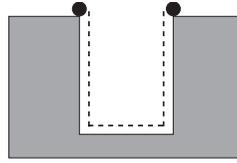
**Creepage is the distance between two points over the surface**
