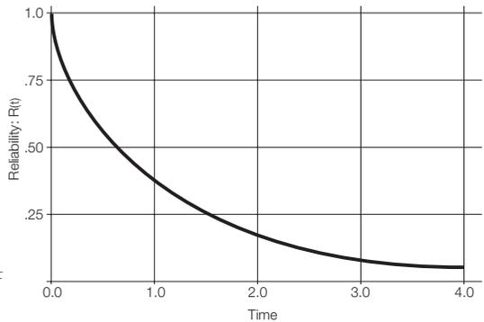
To put these numbers into context, consider a power supply with an MTBF of 500,000hrs (or a failure rate of 0.002 failures per 1000hrs). Using the above equation,  $R(t)$  for 26,280hrs (three years) is approximately 0.95 and if such a unit is used 24hrs a day for three years the probability of it surviving is 95%. The same calculation for a ten year period will give an  $R(t)$  of 84%. If 700 units are used, on average 0.2%/1000hrs will fail, or approximately one per month.
