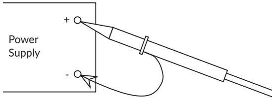
To prepare the probe for high frequency measurement, first remove the clip-on ground wire and the probe body fishhook adapter and then attach a special tip and ground lead assembly as shown in the figure below.
