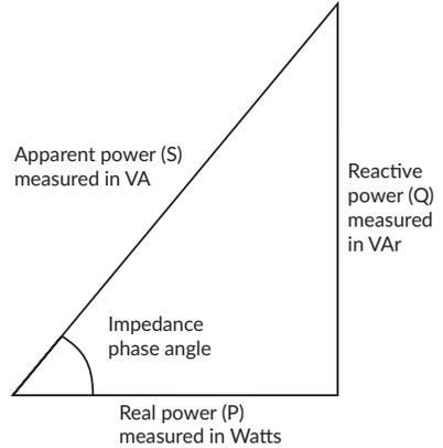
In this form we can see that the opposite angle gives us the impedance of the circuit. Using the cosine of this angle provides the 'power factor' of the circuit.
