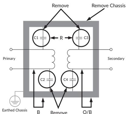
**Power supply disassembly may be required for type testing**
