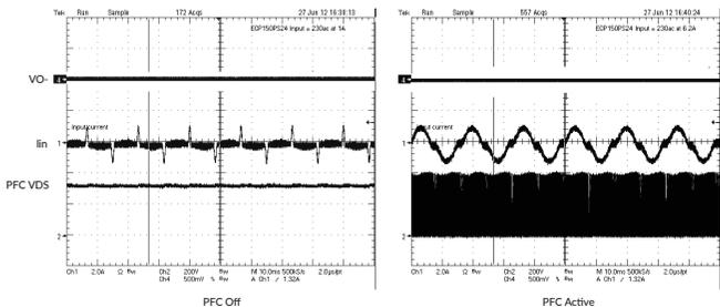
During the on/off transition of the PFC boost converter it may be possible to detect some audible noise.
