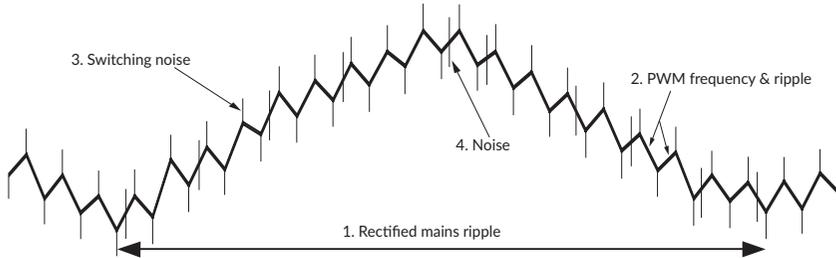
**Typical output ripple and noise trace**
