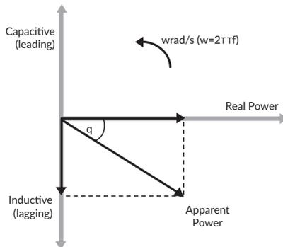
*Phasor diagram of motor load*
