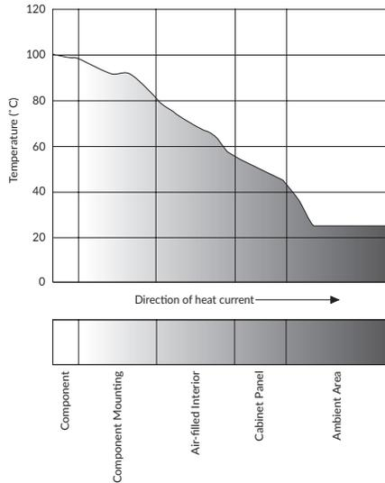
**Temperature gradient of a device to ambient**
