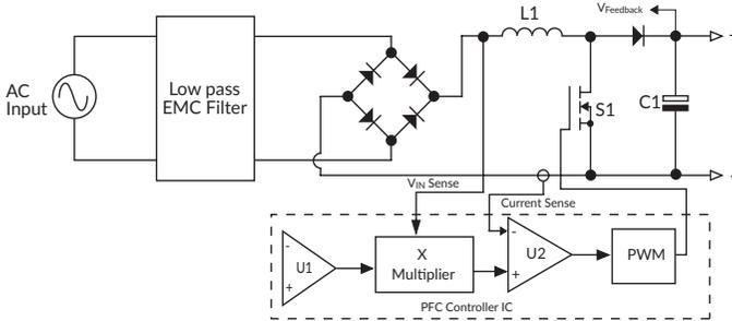
The low pass EMC filter takes the high frequency element and filters it out so that the current seen by the mains supply is sinusoidal. The system regulates the DC output at approximately 400VDC. The diagram below shows real time measurement of active power factor correction.
