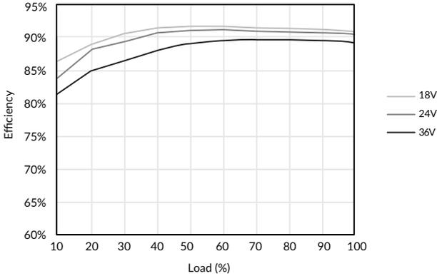
Once the efficiency at the worst-case operating point is established the waste power to be dissipated as heat is calculated as below: -
