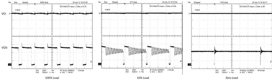
A side effect of burst mode operation can be audible noise at no load or very light load as components with parts which can move under electrical stress can act as transducers and emit audible noise. These may be wound components, filter capacitors, line capacitors & snubber capacitors. This low level audible noise is normal and does not indicate malfunction.
