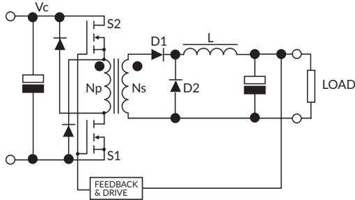
*Two Transistor Forward Converter*
