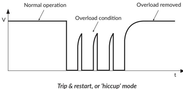
This type of overload limit is generally unsuitable for high inrush loads, such as capacitive loads and lamps or for battery-charging applications which benefit from constant power or constant current characteristics.
