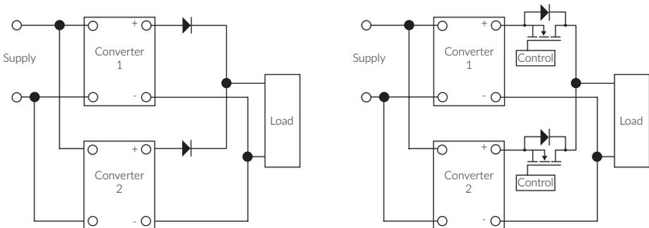
Diodes or MOSFETs can be used in redundant systems so that if one power supply fails the other will continue to operate without the failed power supply pulling down the output rail. Diodes and MOSFETs should always be rated higher than the power supply output current limit.
