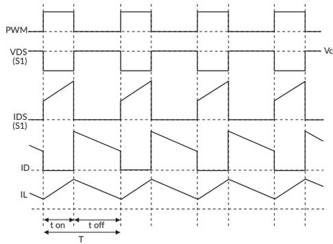
During the switching element on-time the current through the inductor rises as the input voltage is higher than the output voltage and the inductor acquires stored energy. When the switch opens the current freewheels through the diode and supplies energy to the output.
