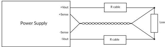
The sense connections monitor and regulate the output at the point of use and adjust the power supply terminal voltage to compensate for variations caused by the impedance of the wiring between the supply and the load. The amount of compensation is typically limited to around 0.5V in total or 0.25V for each of the output & return cables.
