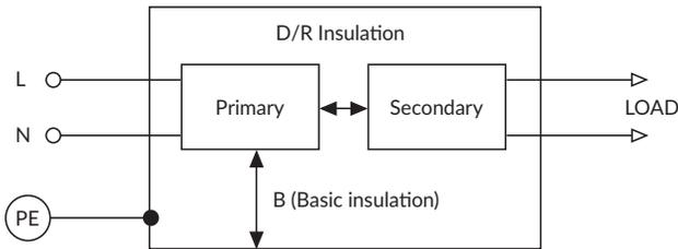
The diagram above represents a complete class I power supply. Primary to earth protection is provided by basic insulation and protective earth (LOP 2). Primary to secondary protection (240VAC to 12VDC) is provided by double/reinforced insulation (Total LOP 2).
