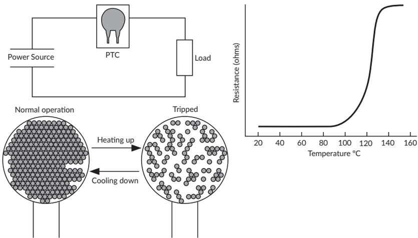
*Resetting PTC thermistor fuse characteristics*
