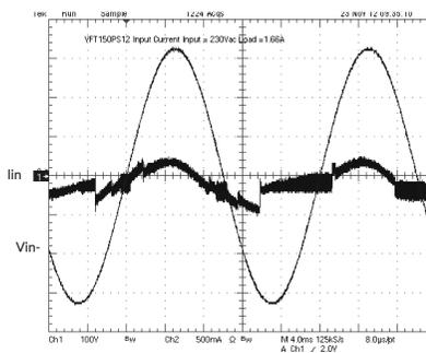
In addition to the non-sinusoidal input current it may be possible to detect audible noise as the boost converter transitions on/off.
