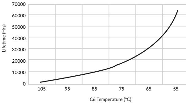
Selecting and evaluating a product such as this, based on the readily available thermal data, rather than one continuously rated for the full peak power results in a smaller, lighter, lower cost solution without compromising the performance, reliability and lifetime of the end application.
