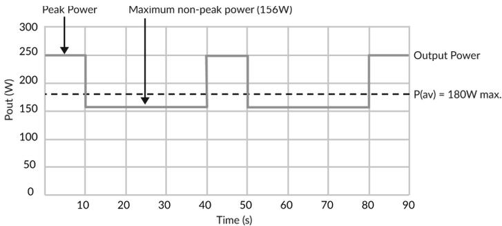
$$P_{av} = \frac{(P_{pk} \times T_1) + (P_o \times T_2)}{T_1 + T_2}$$
