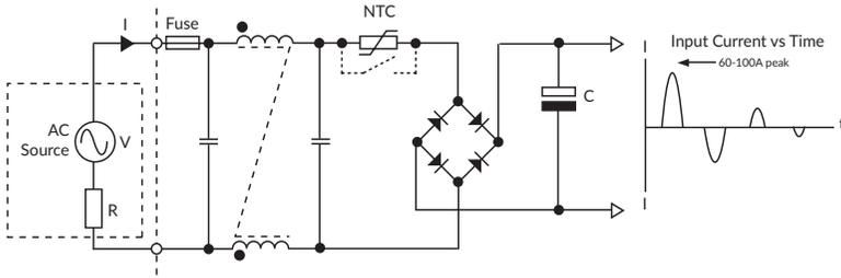
**Typical power supply input circuit**
