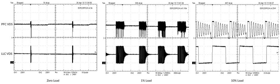
Noticeable effects when using this topology are reduced power factor, non-sinusoidal input current and audible noise from both the PFC boost converter and the LLC resonant converter.
