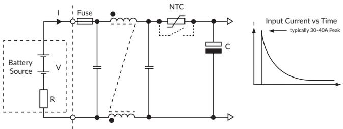
**Typical DC-DC converter input circuit**
