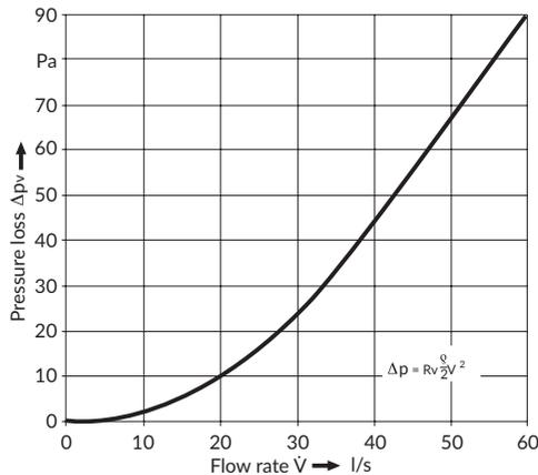
This can be used to estimate the system back pressure, where 1m<sup>3</sup>/hr = 0.278l/s for the example above approximately 10 Pascals.
