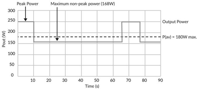
Calculations show that these operating conditions will not exceed the ratings of the power supply. However, we must also consider the key component temperatures of the supply when installed in the unique end equipment to ensure safe, reliable operation over the design life of the end equipment.
