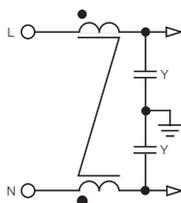
Differential mode noise is attenuated by use of an X capacitor between the line or positive and the neutral or negative in conjunction with a differential mode inductor. Sometimes the differential mode inductor is formed from the leakage inductance of the common mode inductor so that there is only one visible wound component.
