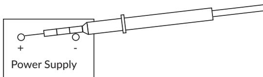
The ground ring of the probe is pressed directly against the output ground of the power supply and the tip is in contact with the output voltage pin.
