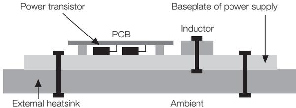
**Basic construction of baseplate cooled PSU with all of the major heat-generating components fixed directly to the baseplate**
