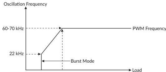
The oscilloscope traces overleaf show the switching waveform and output voltage of a typical 100W green mode component power supply at full load (switching at 62kHz) at 10% load (switching at 35kHz) and at zero load when the supply has entered burst mode to reduce the power consumed to <math><0.5\text{W}</math>. Individual bursts occur at a repetition rate of 900Hz.
