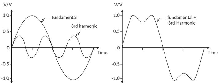
Any waveform that is not sinusoidal contains harmonics. Any distortion or harmonic content will cause the power factor of the system to fall. As with phase shift, any power not being dissipated as useful power to the load is known as reactive power. The effects of harmonic currents within a system cause a reduction in power factor and therefore reduce the efficiency of energy transfer from source to load.
