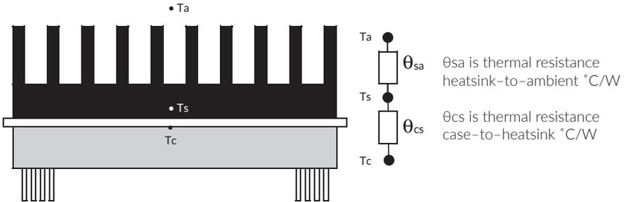
Thermal resistance to the flow of heat from the power module to the ambient temperature air surrounding the package is made up of the thermal resistances of the case to heatsink and heatsink to ambient interfaces and can be added together to give an overall thermal resistance from power module to ambient  $\theta_{ca}$ .
