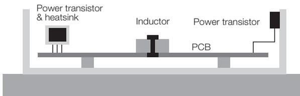
**Construction of typical industrial AC-DC power supply**
