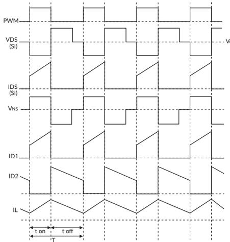
There is no energy stored in the transformer; energy is stored in the output stage of the converter in the inductor and capacitor. The output inductor reduces the ripple currents in the output capacitor and the volume of the transformer is dependent on switching frequency and power dissipation.
