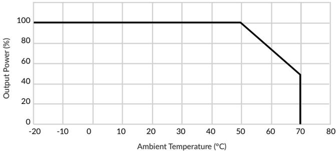
For external plug top and desk top power supplies the de-rating normally starts at 40°C as these products are not exposed to temperature rises within the end equipment.
