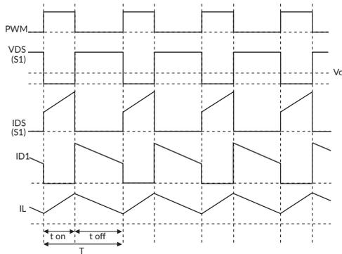
Energy is stored in the inductor during the switching element on-time, the voltage across the inductor is added to the input voltage and transferred to the output capacitor during the switching element off-time. Practically, output voltages of up to five times the input voltage can be achieved.
