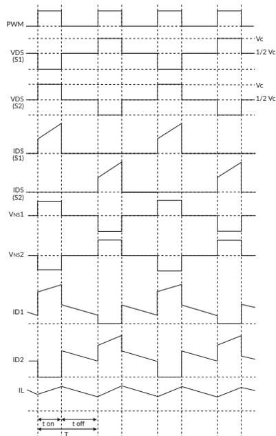
Energy is transferred to the secondary and the load during each switching element on-time by utilizing a split secondary winding. This has the added benefit of doubling the switching frequency seen by the secondary, helping to reduce the volume of the output inductor and capacitor required and halving the voltage seen by each switching element.
