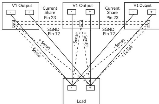
The current share connection interfaces with each power supply comparing the output current and adjusting the output voltage of individual until the current is equally distributed. This sharing interface is ideal for scalable power systems and may be deployed in redundant power systems if it is considered a low enough risk to system fault tolerance.
